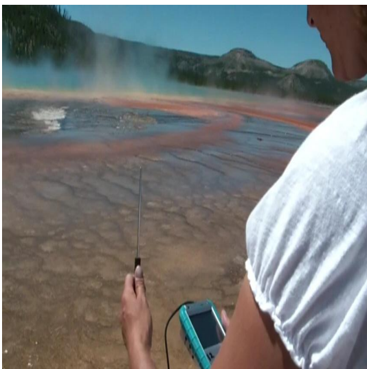
Using the LabQuest to record temperature at the Grand Prismatic Spring
